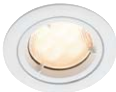
Low Energy twist front fixed downlight complete with 11 Watt GU10 CFL downlight in white Depth 105mm Dia 80mm
