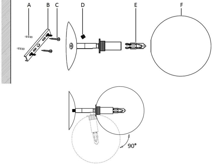
NOTE: When adjusting the wall bracket, do not adjust more than the angle shown above as this may damage the internal wires
