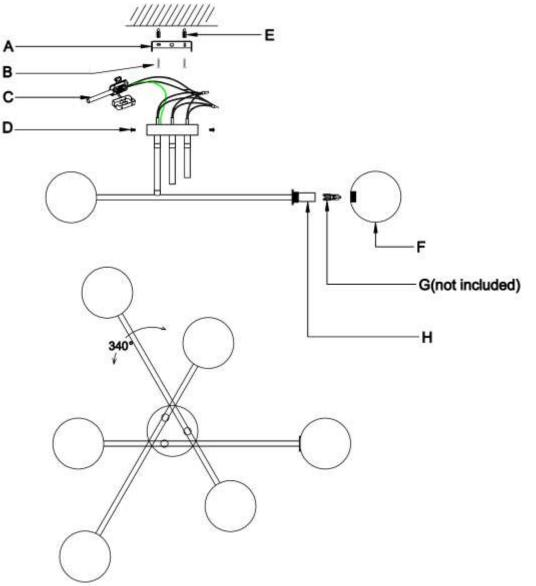
NOTE: When adjusting the arms of the fitting, do not adjust more than 340° as this may damage the wiring. Safety Tips
