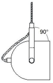
NOTE: When adjusting the shade, do not adjust more than 90° as this may damage the wiring.
