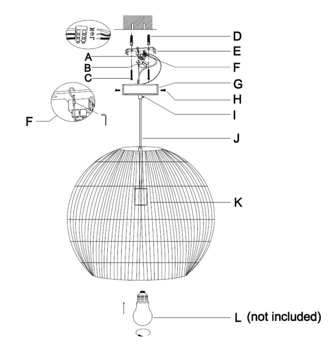
NOTE: The full load/weight of the pendant must always be on the safety lanyard (F) and never on the cord suspension (J).
