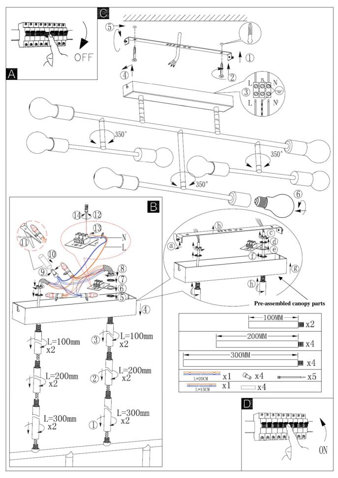
NOTE: Do not rotate the arms more than 350° as this may damage the joint or damage the internal wiring
