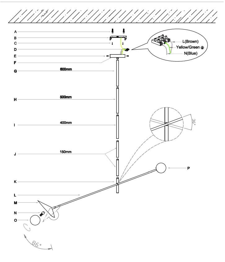
NOTE: Do not adjust the arm (L) more than 36°, as this may damage the joint or the internal wiring. NOTE: Do not adjust the head (M) more than 86°, as this may damage the joint or the internal wiring.
