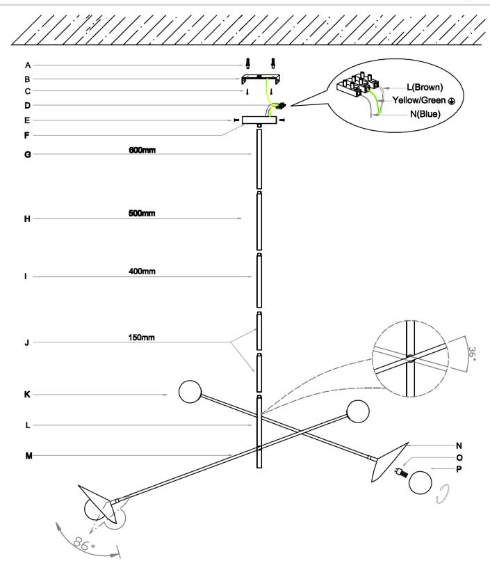
NOTE: Do not adjust the arm (M) more than 36°, as this may damage the joint or the internal wiring. NOTE: Do not adjust the head (N) more than 86°, as this may damage the joint or the internal wiring.
