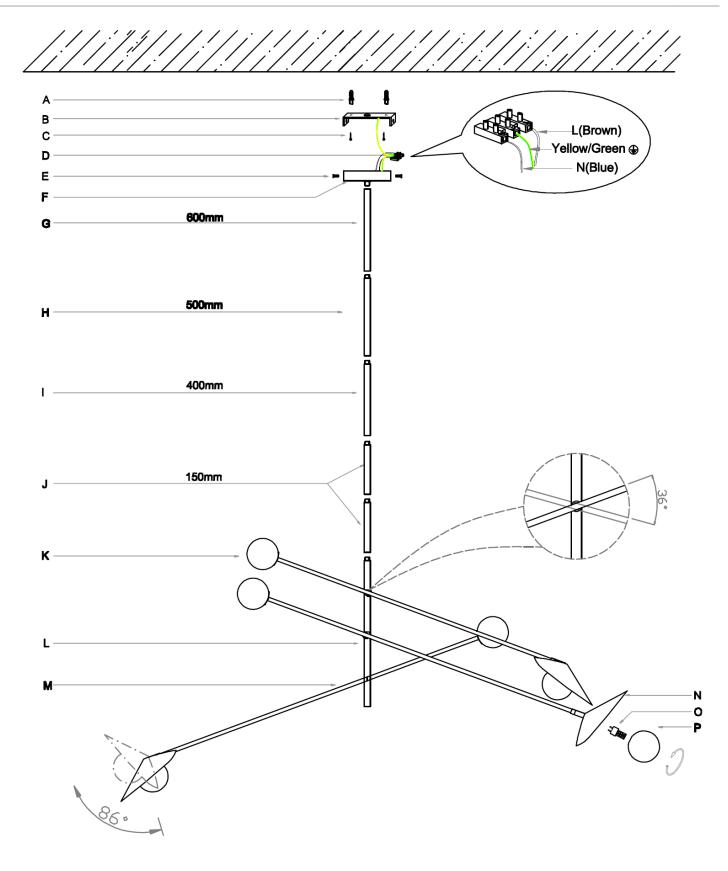
NOTE: Do not adjust the arm (M) more than 36°, as this may damage the joint or the internal wiring. NOTE: Do not adjust the head (N) more than 86°, as this may damage the joint or the internal wiring.
