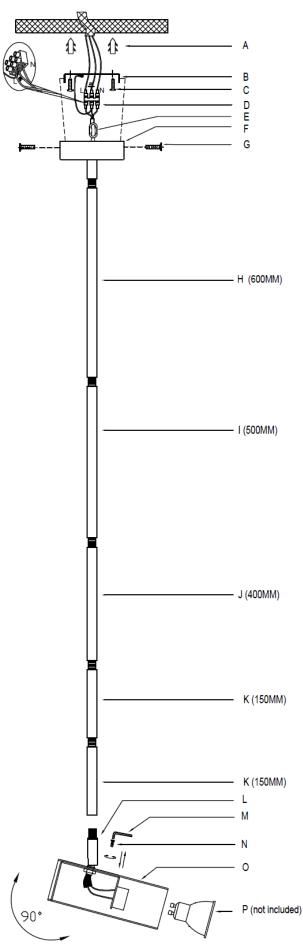
NOTE: Do not adjust the head (O) more than  $90^{\circ}$ , as this may damage the joint or the internal wiring.
