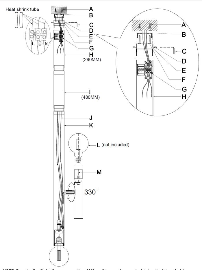
NOTE: Do not adjust/twist the arm more than 330°, as this may damage the joint or the internal wiring.
