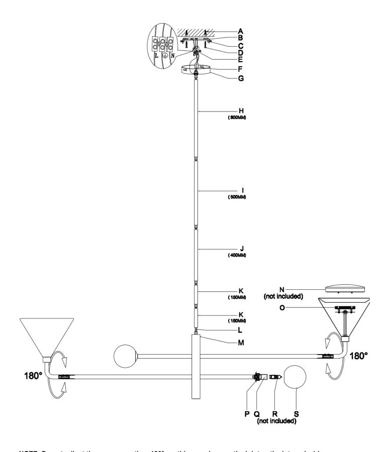
NOTE: Do not adjust the arms more than 180°, as this may damage the joint or the internal wiring.
