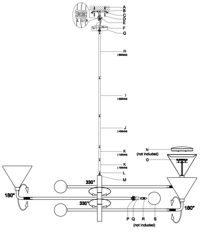
NOTE: Do not adjust the heads more than 180°, as this may damage the joint or the internal wiring. NOTE: Do not adjust the arms more than 330°, as this may damage the joint or the internal wiring.
