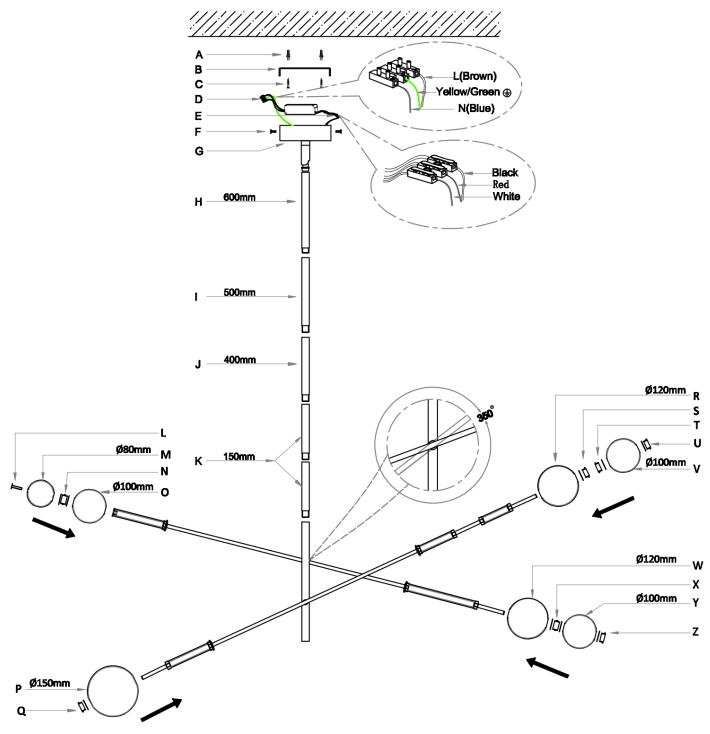
NOTE: Do not adjust the arms more than 350°, as this may damage the joint or the internal wiring.
