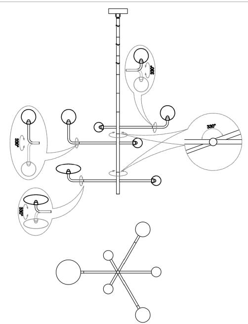
NOTE: Do not adjust the arm and shade more than 330°, as this may damage the joint or the internal wiring.
