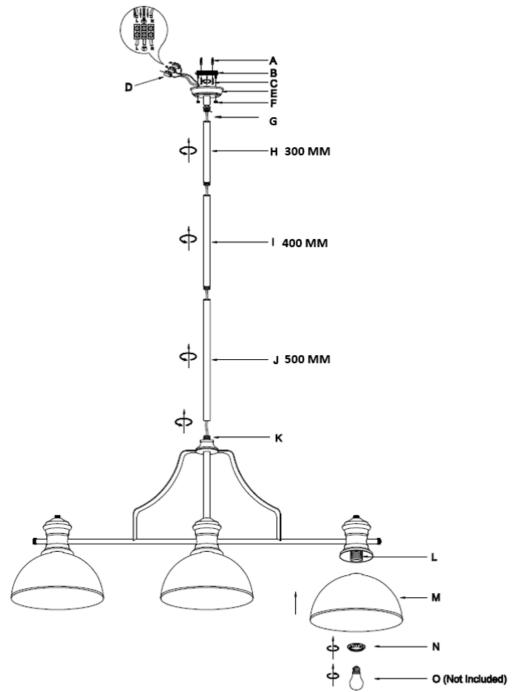
**NOTE:** A minimum clearance of 0.5m must be kept between the fitting and any walls or building elements when it is installed on the ceiling with a pitch angle. (Refer to the specification table for the maximum pitch angle).
