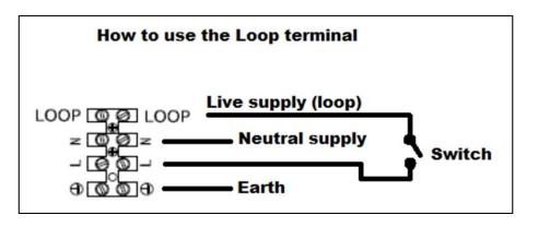
NOTE: If you are using the LOOP TERMINAL, please ensure the loop terminal is covered.
