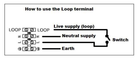
NOTE: Must Install the terminal block cover (H) back onto the terminal block (G).
