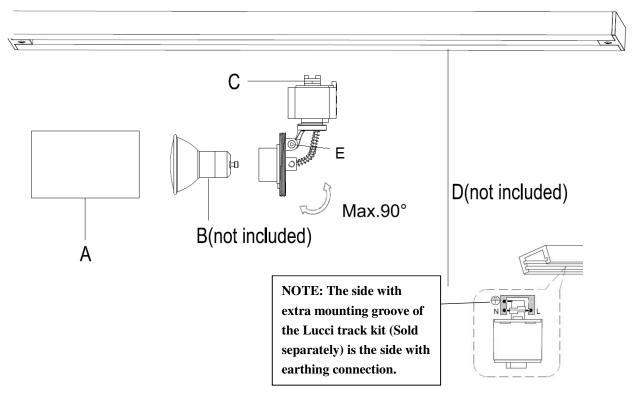
NOTE: Do not adjust light head over 90° to the horizontal which can damage the internal wires.
