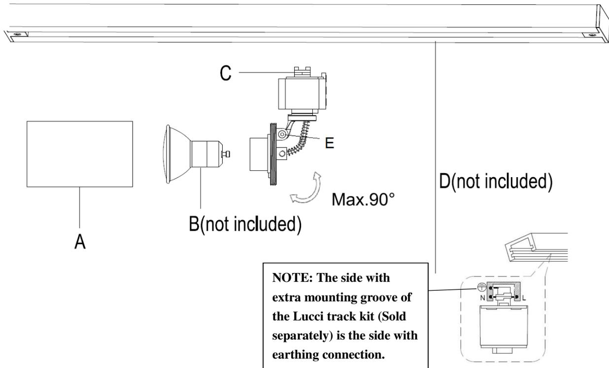
**NOTE: Do not adjust light head over 90° to the horizontal which can damage the internal wires.**
