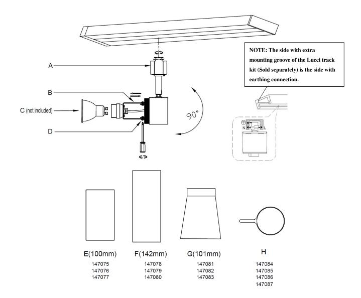
NOTE: DO NOT adjust light head over 350° horizontally and 90° vertically which can damage the internal wires.
