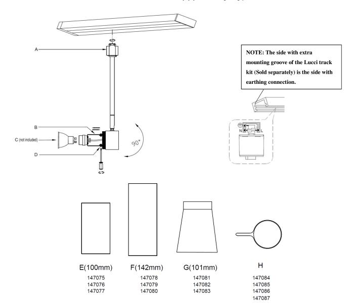
NOTE: DO NOT adjust light head over 350° horizontally and 90° vertically which can damage the internal wires.
