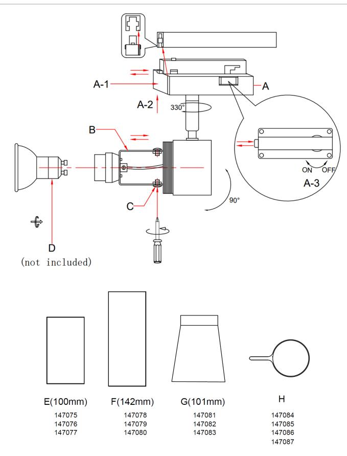
NOTE: DO NOT adjust the head up or down more than 90° and DO NOT rotate the head more than 330°. As this may damage the knuckle joint and the internal wires.
