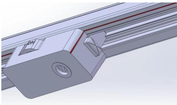
8. Check and ensure the lock on the track adaptor (A) is in the “OFF” position.
