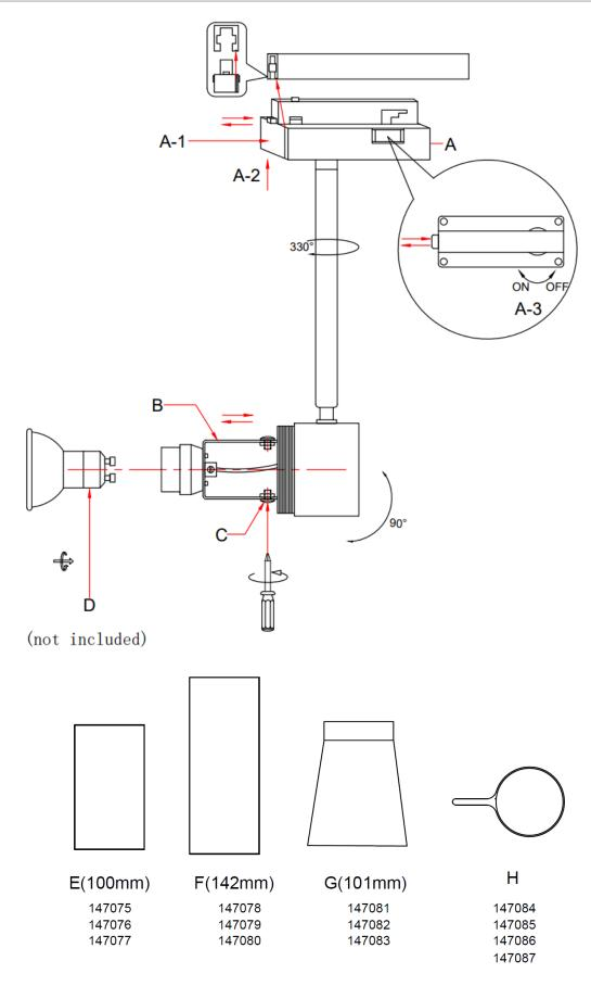
NOTE: DO NOT adjust the head up or down more than 90° and DO NOT rotate the head more than 330°. As this may damage the knuckle joint and the internal wires.
