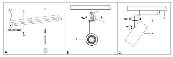
**NOTE:** When adjusting the lamp head (4), do not rotate more than 350°, or raise upward more than 90°, as this may damage the internal wiring.
