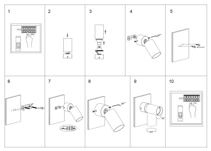
NOTE: Do not bend the spot head more than 90° as this may damage the internal wiring.
