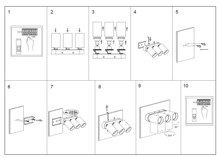
NOTE: Do not bend the spot heads more than 90° as this may damage the internal wiring. NOTE: Do not rotate the spot heads more than 350° as this may damage the internal wiring.
