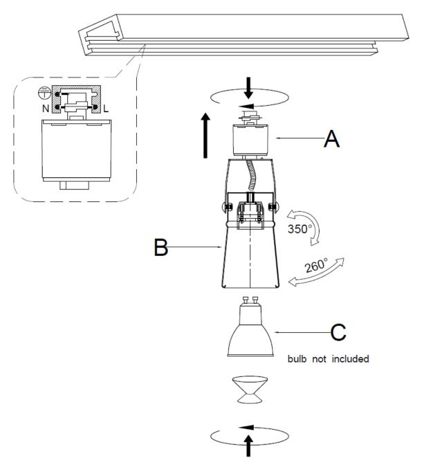
NOTE: When adjusting the spot lights, do not adjust more than the angles showed in the figure as this may damage the wiring.
