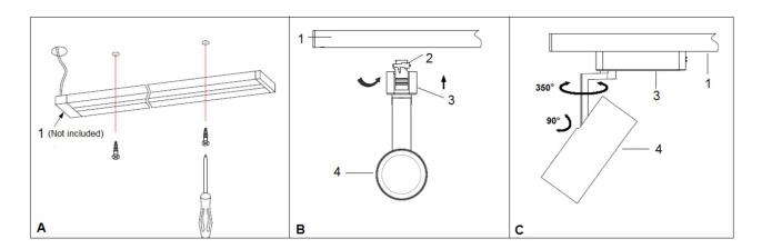
NOTE: When adjusting the lamp head (4), do not rotate more than 350° or 90° in either direction shown, as this may damage the internal wiring.
