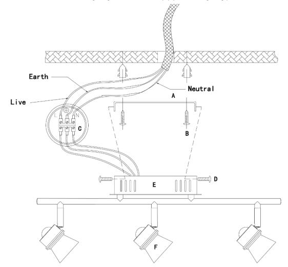
NOTE: Do not bend the spotlight (F) up and down more than 90° and do not rotate the spotlight (F) more than 350° as this may damage the knuckle joint or damage the internal wiring.
