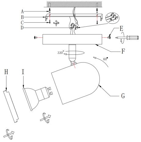
NOTES FOR ARM AND SHADE ADJUSTMENT: To avoid and damage to the joints or internal wiring, please do not adjust the arm or shade (G) beyond the angles listed:
