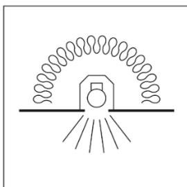
1. Type IC recessed luminaire can be used together with building insulation that can safely be exposed continuously to temperatures up to 90°C may abut and cover the luminaire.
