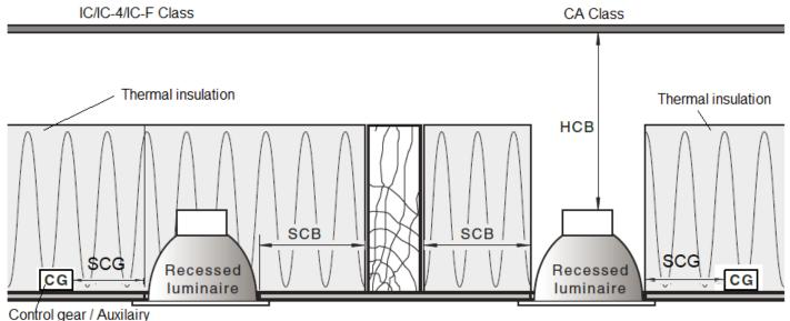
equipment driver / transformer (Control gear of this luminaire can be placed under thermal insulation)
