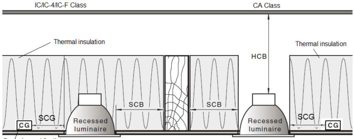
Control gear / Auxilairy equipment driver / transformer (Control gear of this luminaire can be placed under thermal insulation)
