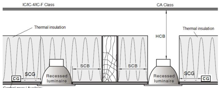
Control gear / Auxilairy equipment driver / transformer (Control gear of this luminaire can be placed under thermal insulation)
