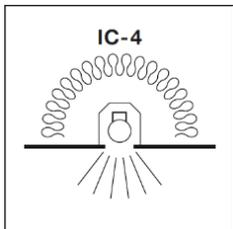
A recessed luminaire that can be abutted against normally flammable materials, including building insulation, and can be covered in normal use. Building elements and building insulation to the heated parts of the luminaire. This classification of recessed luminaire is effectively a sealed unit that has a restricted flow of air between the habitable room the luminaire emits light into and the void/space where the main body of the luminaire is located.
