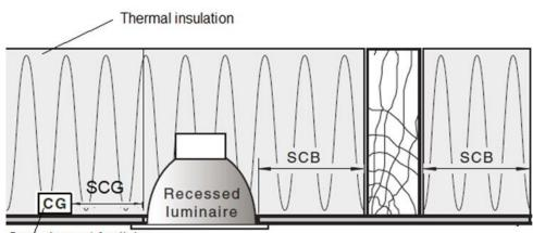
Control gear / Auxilairy equipment driver / transformer (Control gear of this luminaire can be placed under thermal insulation)
