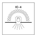
1. A closed luminaire that allows building insulation to come into contact with its sides and to cover it.
