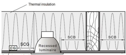
Control gear / Auxilairy equipment driver / transformer (Control gear of this luminaire can be placed under thermal insulation)
