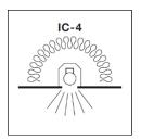
A recessed luminaire that can be abutted against normally flammable building materials, including building insulation, and can be covered in normal use. Building elements, building insulation or debris have restricted access to the heated parts of the luminaire. This classification of recessed luminaire is effectively a sealed unit that has a restricted flow of air between the habitable room the luminaire emits light into and the void/space where the main body of the luminaire is located.
