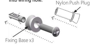
1D Connect the assembled rail onto the Fixing Bases and Nylon Push Plug on the wall.
