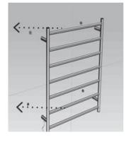
drill holes in marked positions and mount fixing bases into the wall using Mounting Screws and plastic expanders.
