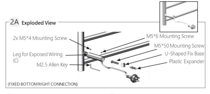
Attach legs to the towel rail & mark the desired location onto the wall as per the measurements on Page 3
