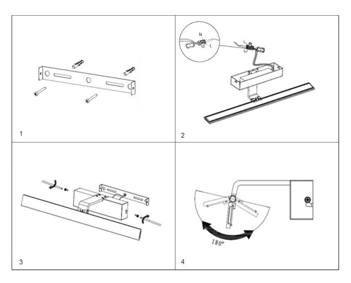
NOTE: Do not adjust head more than 180 degrees as this may damage the internal wires.
