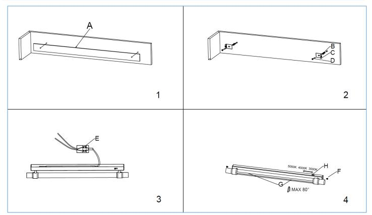
NOTE: Power to the luminaire must be turned OFF, before sliding the switch to select the colour temperature. NOTE: When adjusting the angle, do not rotate more than 80° as this may damage the internal wiring.
