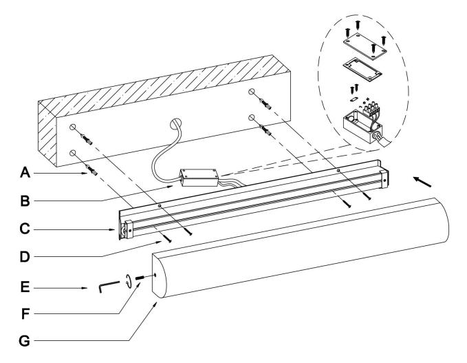
NOTE: Install the grub screws (F) until they are flush with the shade (G) and the shade is secure. NOTE: Do not overtighten the grub screws (F) as it will crack and damage the shade (G).
