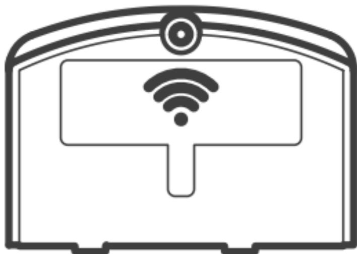
Loosen the screw and remove the cover.
