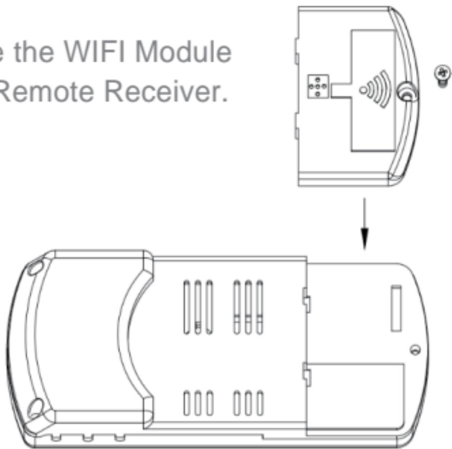
Secure it by tightening the screw.
