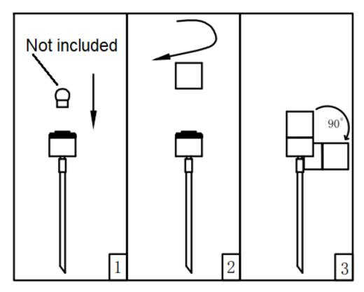
NOTE: Do not adjust the head more than 90°, as this may damage the joint or the internal wiring.
