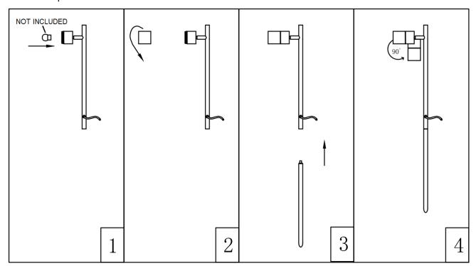
NOTE: Do not adjust the head more than 90°, as this may damage the joint or the internal wiring.
