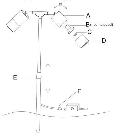
NOTE: Do not adjust the spot heads (A) more than 90°, as this may damage the joint or the internal wiring.
