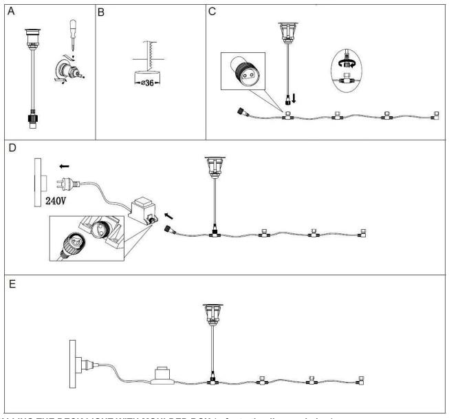
INSTALLING THE DECK LIGHT WITH MOULDED BOX (refer to the diagram below)
